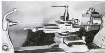
Using the indicator to center a punch mark in an irregularly shaped casting prior to boring
